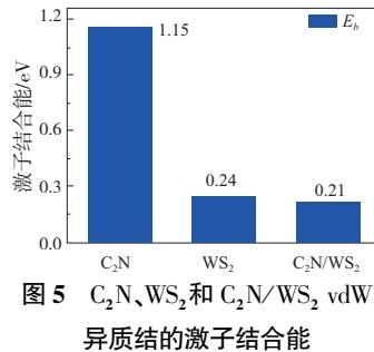
图 5 C<sub>2</sub>N, WS<sub>2</sub> 和 C<sub>2</sub>N/WS<sub>2</sub> vdW 异质结的激子结合能
